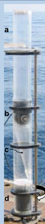
Figure 1. IRS SV Sediment Trap depicting the (a) particle interceptor, (b) indented rotating sphere, (c) funnel that feeds into sample collection cups, and (d) carousel housing the sample collection cups.
