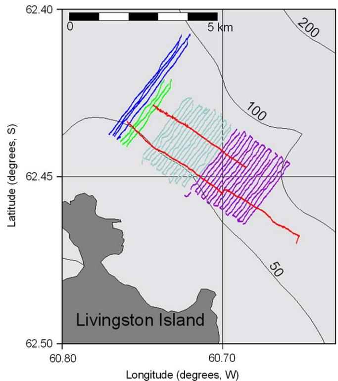
**Fig. 1.** The Cape Sheriff study site, Livingston Island, South Shetlands, Antarctica. Multi-beam survey transects are shown, colour coded by day. Bathymetric contours are shown as black lines. Note the two tie-lines which were surveyed perpendicular to the main survey.
