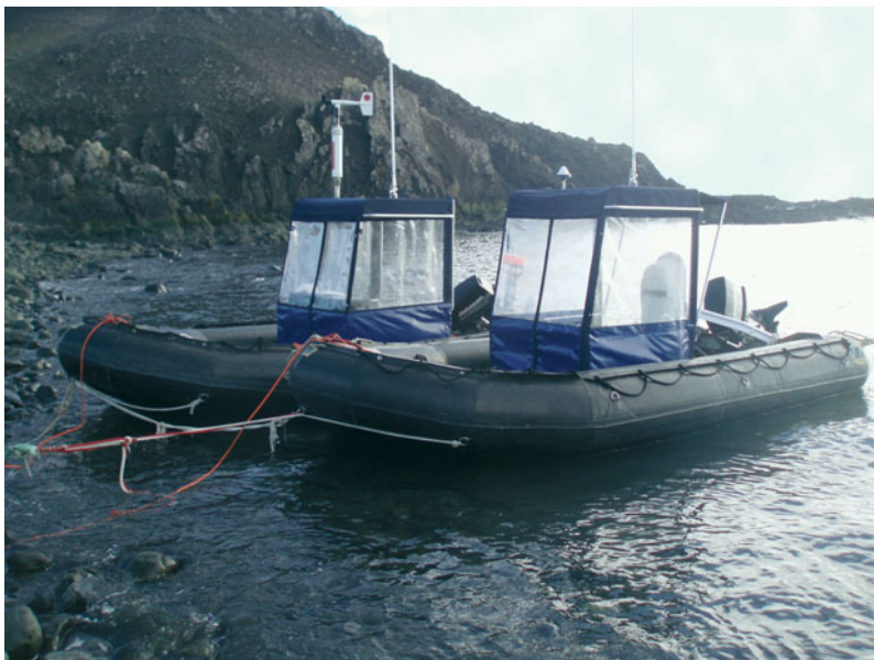
Fig. 3. The MBE-equipped RV 'Roald' (right-hand vessel) and single-beam echosounder (SBE)-equipped RV 'Ernest'. The MBE blister fairing (white) was mounted on a rotating frame attached to the Zodiac's transom (it is visible in the 'up' position through the transparent side of the dodger)
