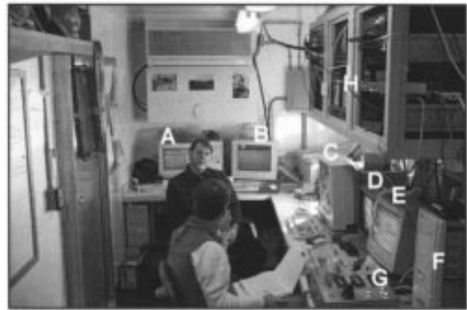
Fig. 5. Interior of the control van during a BIOMAPER-II survey in the Gulf of Maine—Peter Wiebe (facing camera) and Charles Greene. (A) BIOMAPER-II engineering status computer display. (B) Post-processing computer display. (C) Digital echo sounder display. (D) Deck camera display. (E) Environmental sensor computer display. (F) VPR processing computer. (G) Moveable winch controller box. (H) Instrument rack.
